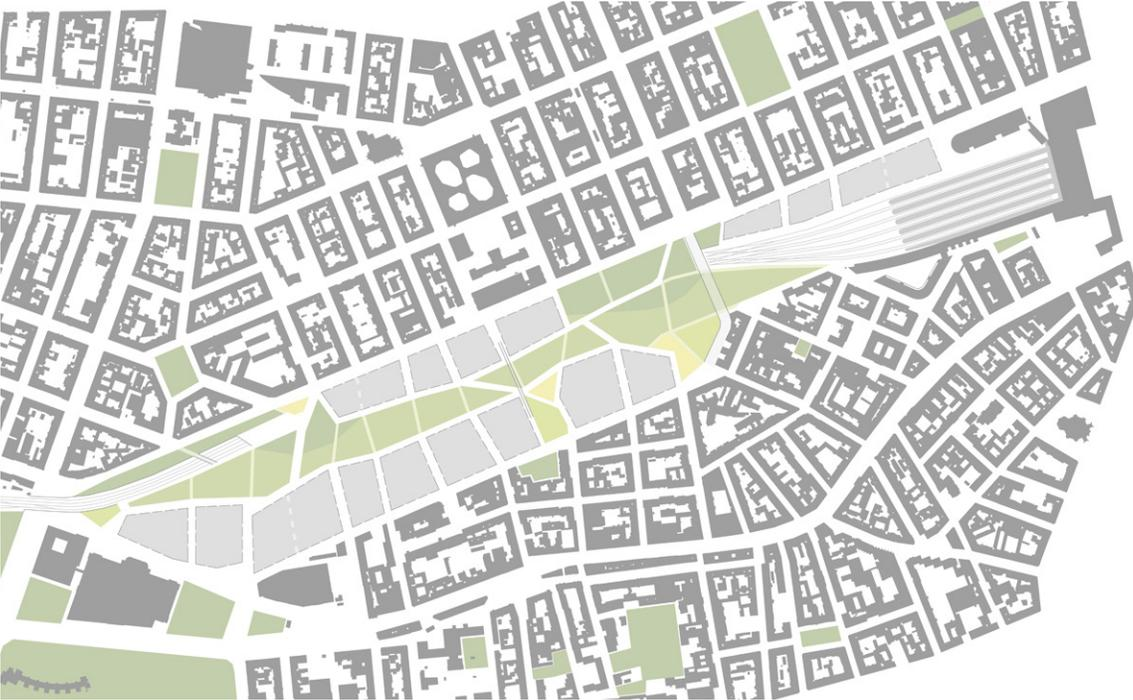
Fig. 10: Site Plan, the Block size provides frequent route choice, park provides cooling
