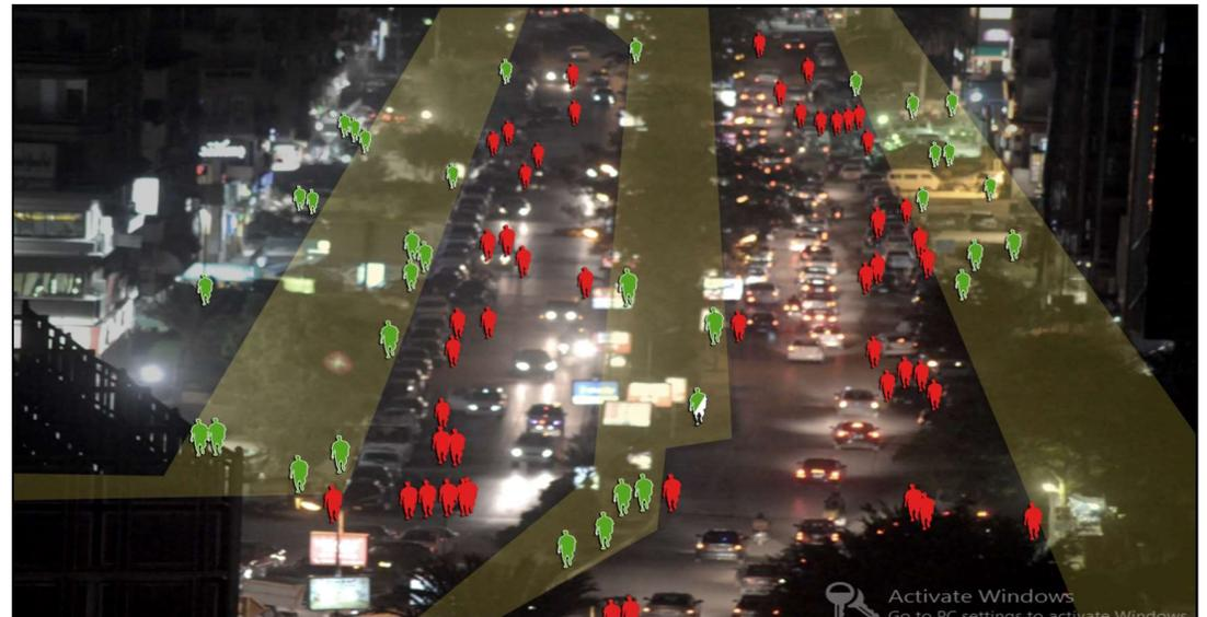
2) A 2.0 m wide lane of cars permanently park attached to sidewalks. Thus, this lane of parking cars enhances the disconnectivity of sidewalks.
