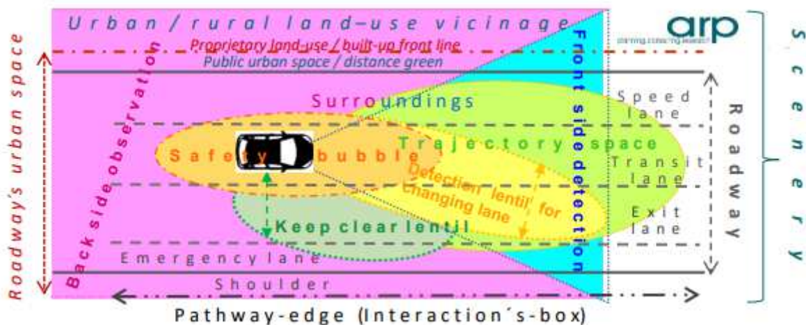
Figure 2: Fields of vision detected by a solitary car to claim a trajectory onto his pathway
