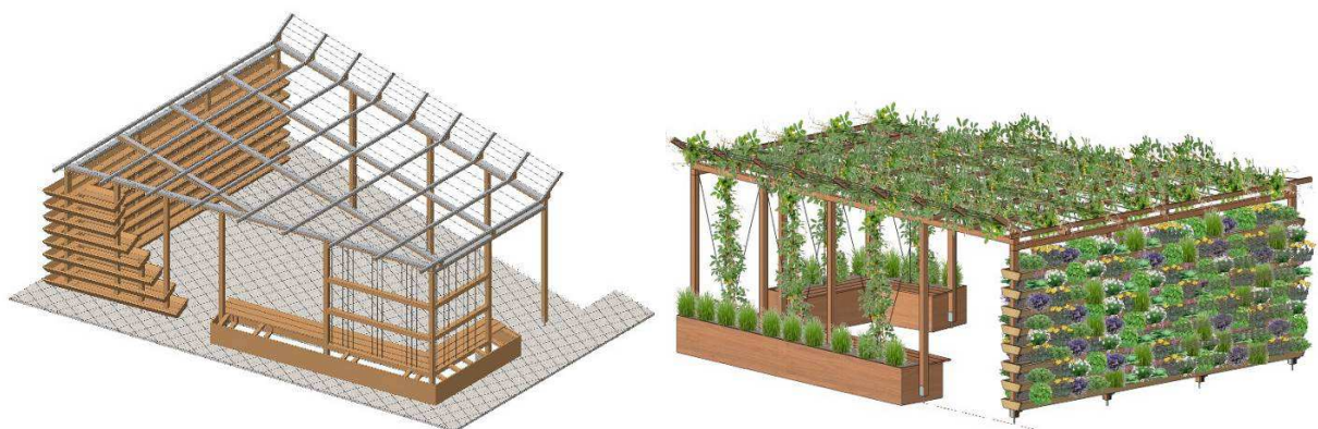
Fig. 6 and 7: Construction details and visualisation of a draft of the outdoor classroom with EVAPO+ transpiring green wall
