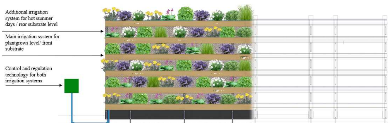
Fig. 2: Separate water circuits for watering the EVAPO+ transpiring green wall on the roof terrace of the Strasshof municipal office building
