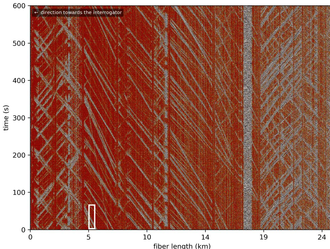
Fig. 2: Image representation of FOAS signal spectral power produced from raw FOAS data, showing vehicle trajectories on a highway over 25 km length. The y-axis represents the time, the x-axis the position along the fiber cable length.
