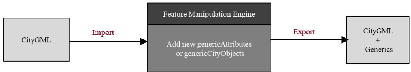
Fig. 1: A typical workflow to extend CityGML with generics using FME
