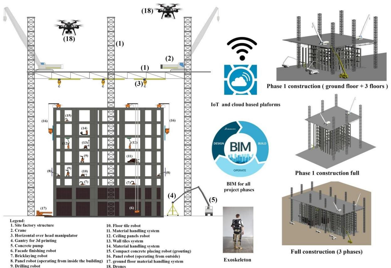
Fig. 32: Building construction progress, robots, systems and technologies used for automation (Researchers, 2021)
