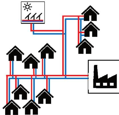
Fig. 1: Schematic overview showing the basic parts of a DHS according to its fundamental idea.
