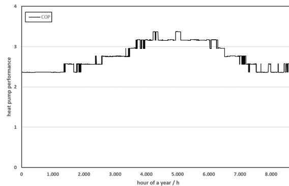
Fig. 10: Performance of chosen river water heat pump.
