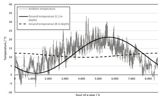
Fig. 8: Ground temperatures calculated from the ambient temperature.
