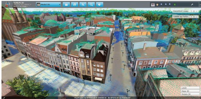
Fig. 8: Combining detailed building models of historical centre of Toruń with LIDAR point clouds, 3D module of Toruń's City geoportal.
