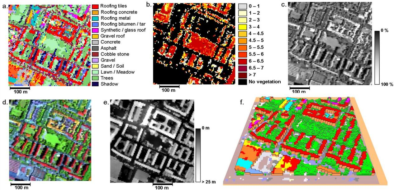
Figure 4: Input data for the micro climate model ENVI-met. Upper line: maps derived from the HyMap data: surface materials (a), leaf area index (b) and albedo (c). Lower line: the HyMap subset (d) and DEM subset (e) of the study area and the final 3-D input file for the model (f).
