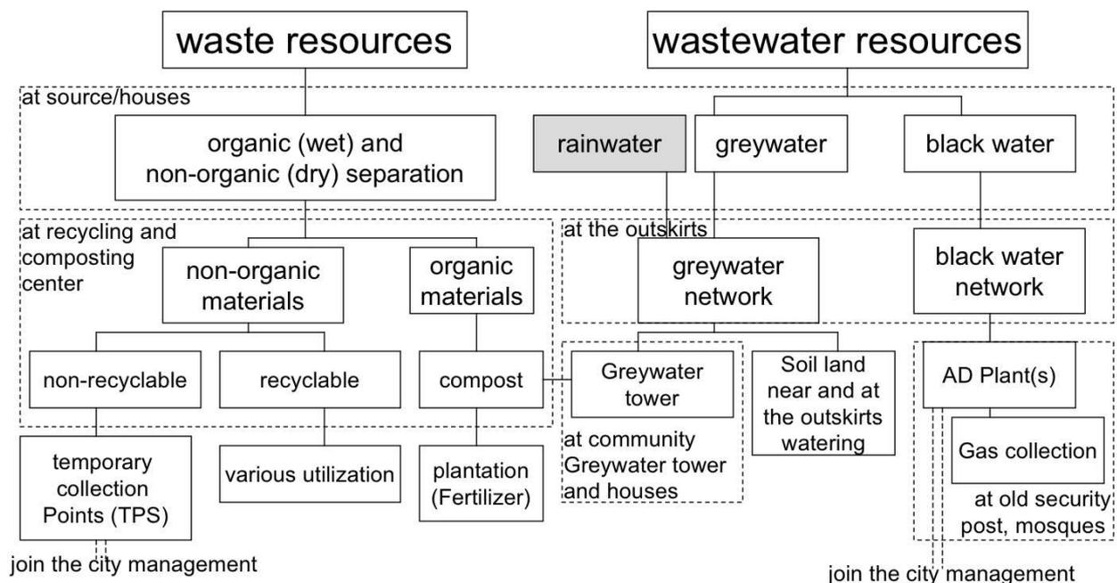
Note: Rainwater is not included as wastewater but however it joins greywater network to for utility
