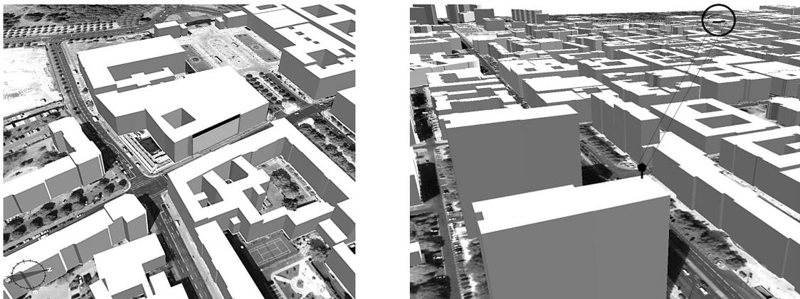
Fig. 8: 3D visibility analysis within the virtual city model using the example of the British embassy (left, building within the circle). An observer placed on a multi storey building approx. 1.3 km away can just see a small strip on the upper front façade (right, black pigmented rectangle).
