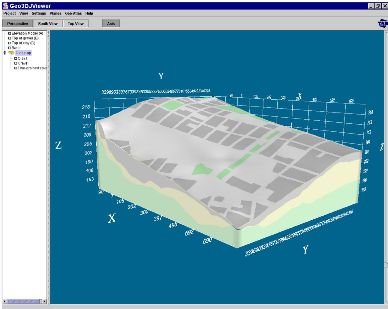
Fig. 5: Close-up view of the geological layer model in the central part of Vienna
